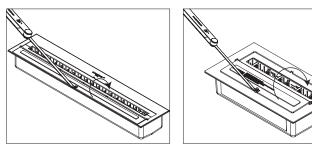
**AB Series and VB Series:** A lid is used to extinguish the flame.
